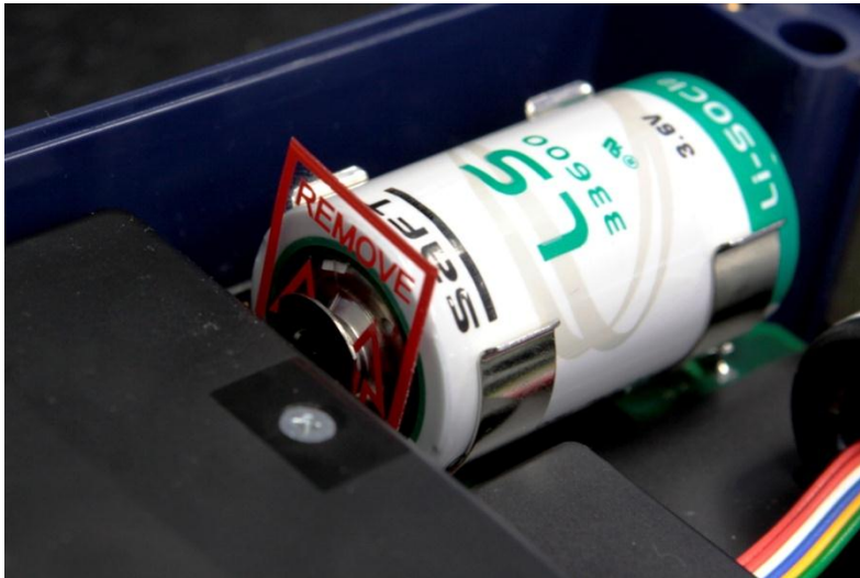
Fig. 13 Removable foil strip in the battery holder
